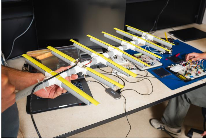
Figure 4: DIY Yagi Antenna for 70cm Band.
