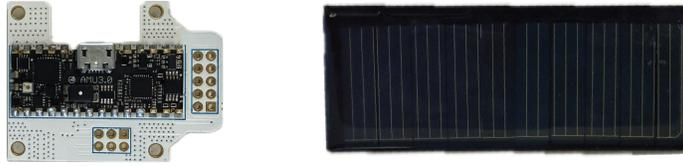
Figure 3: Aerospace Measurement Unit (left) and Solar Cell (right).
